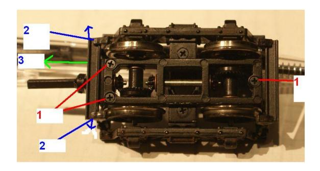
Replace all of the gears indicated by the red lines. Replace any drive lines that have cracked gears.
