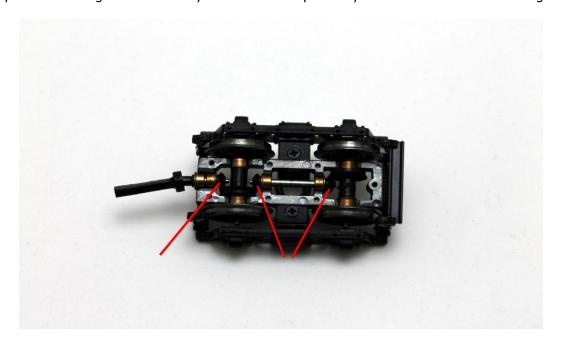
Lube with gear oil as needed.
